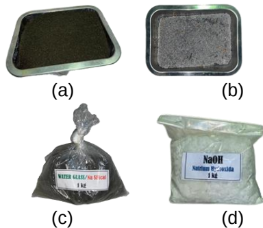
Figure 2. The materials of the experiment: (a) fine aggregate, (b) rice husk ash, (c) Na 2 SiO 3 , and (d) NaOH
